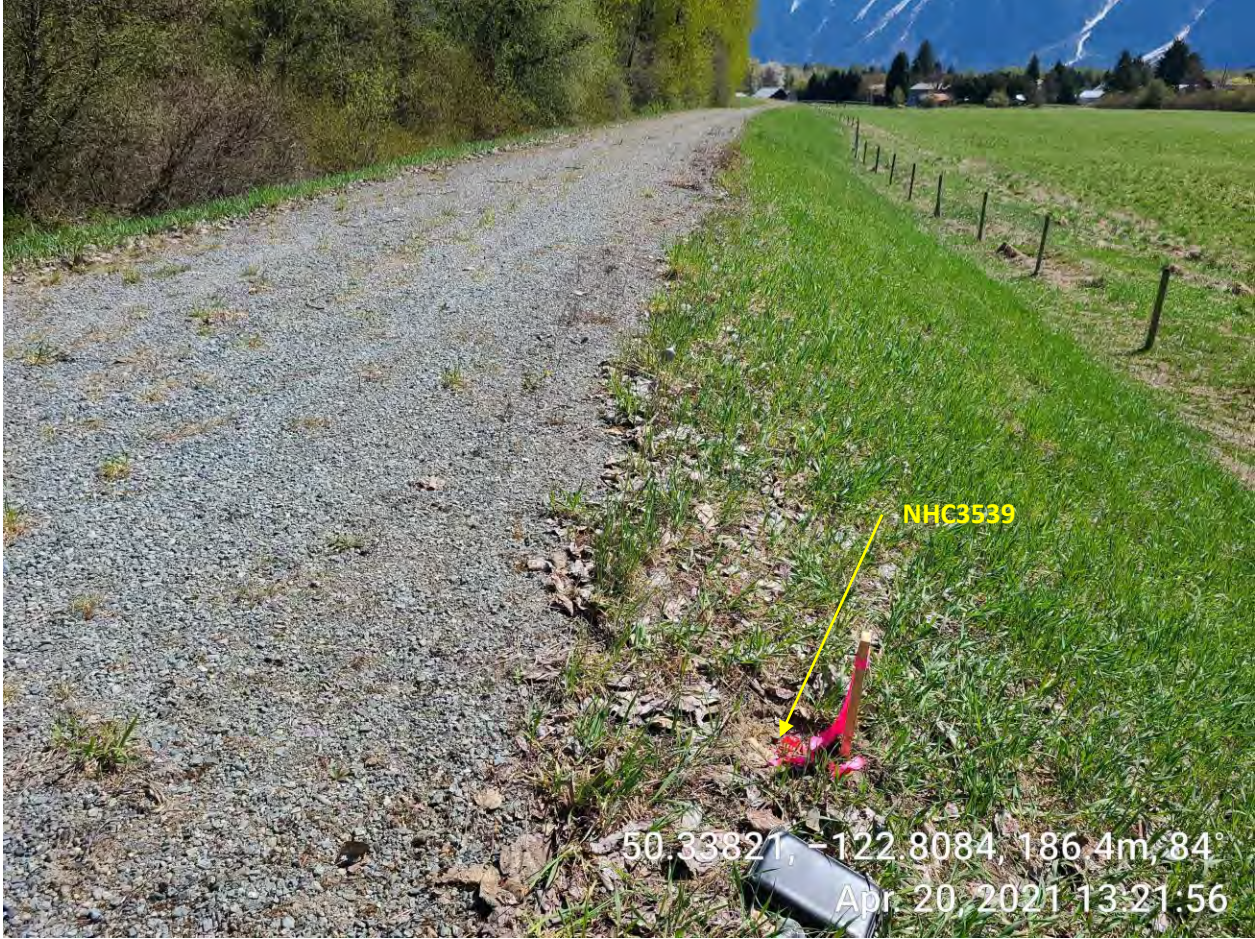
Photo 4 Primary benchmark NHC3539 on top of placed rebar
