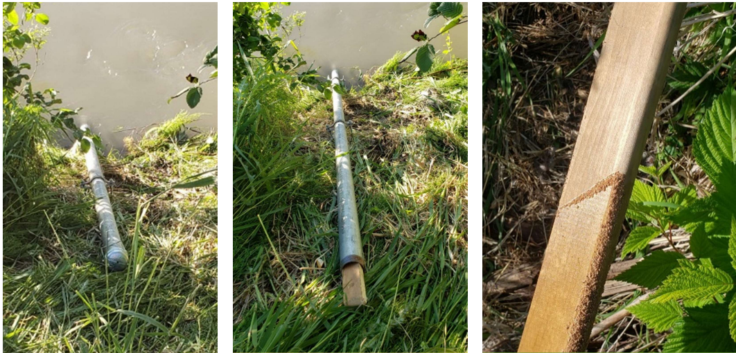
Photo 2.2 From left to right: Installed crest stage gauge; crest stage gauge with inner wood staff extending out; high water mark on wood staff left by cork.
