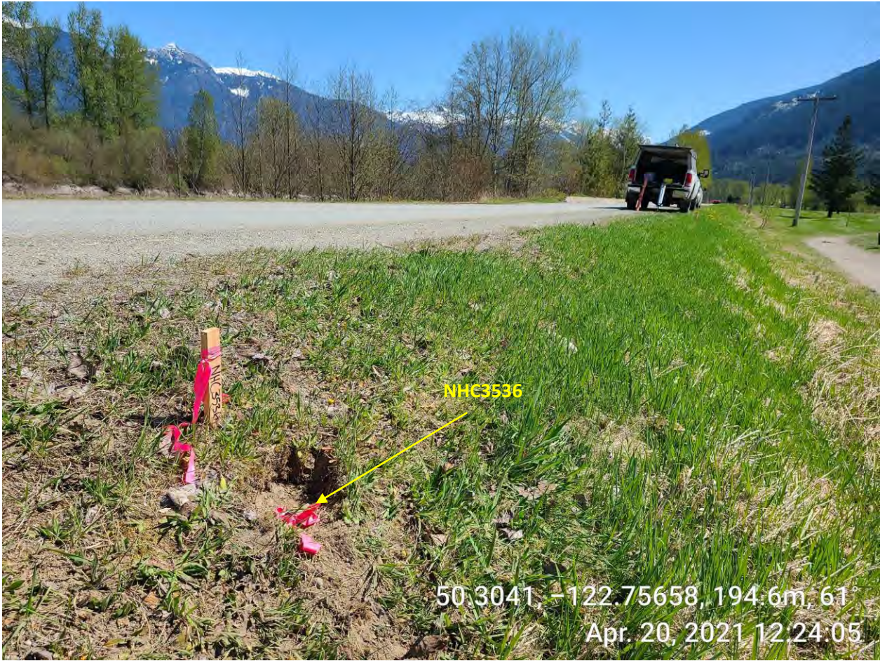
Photo 4 Benchmark NHC 3536 on top of placed rebar
