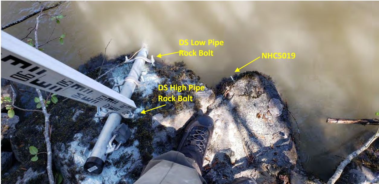
Photo 2 Low Benchmark NHC5019 on rock bolt near pressure transducer pipe.
