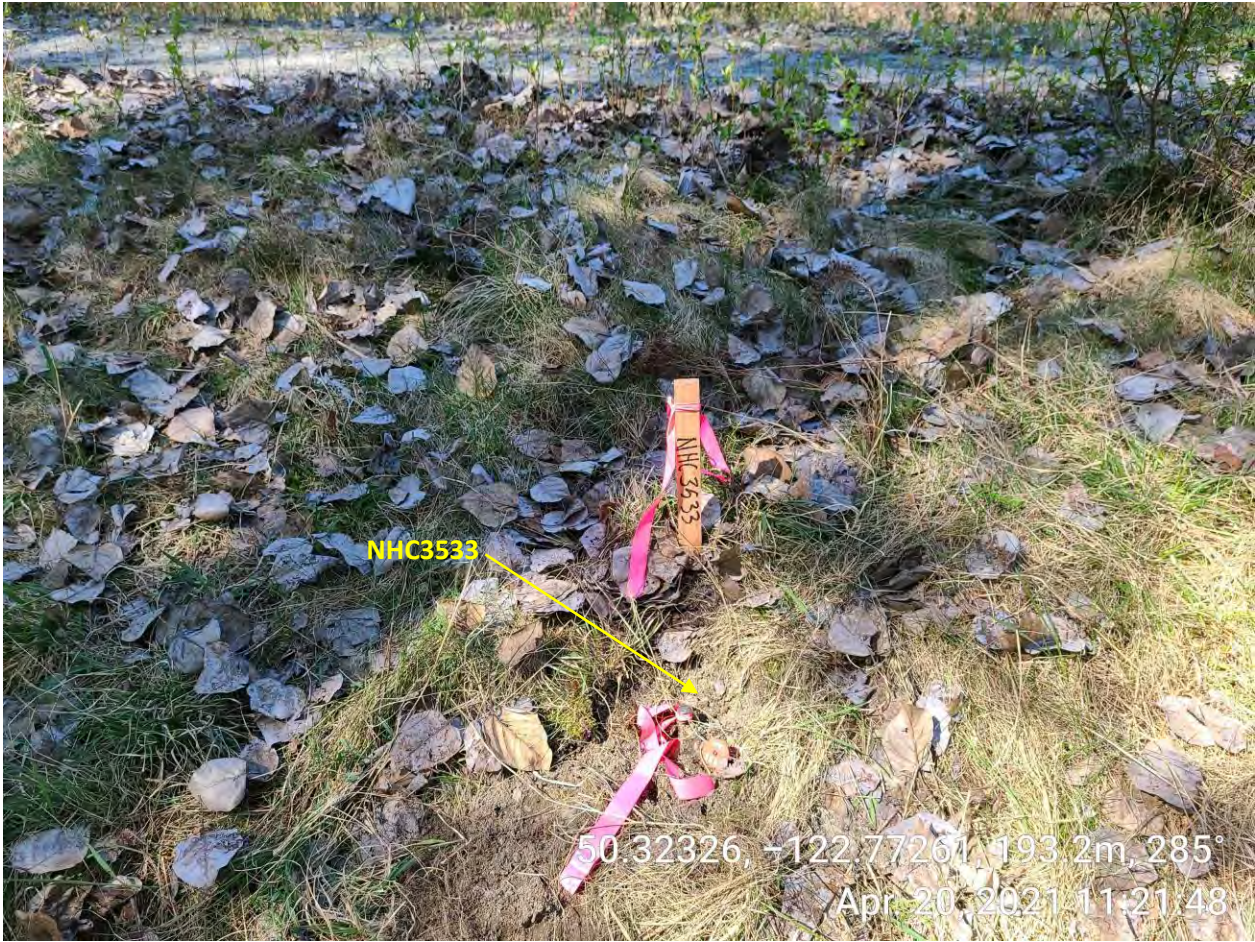
Photo 3 Primary Benchmark NHC3533 on top of placed rebar on dike.
