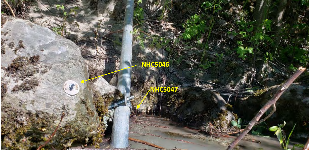
Photo 4 Benchmarks NHC5046 and NHC5047 at Crest Gauge pipe.
