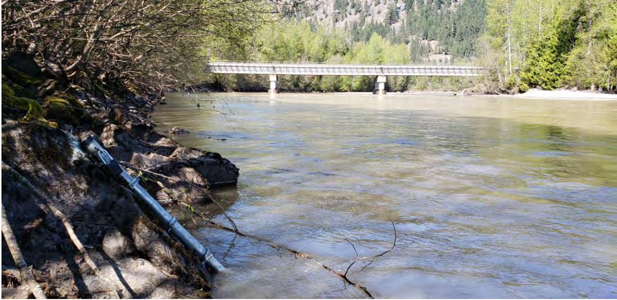
Photo 1 PT stilling well at Lillooet River downstream of Beam Bar (2021-04-19)
