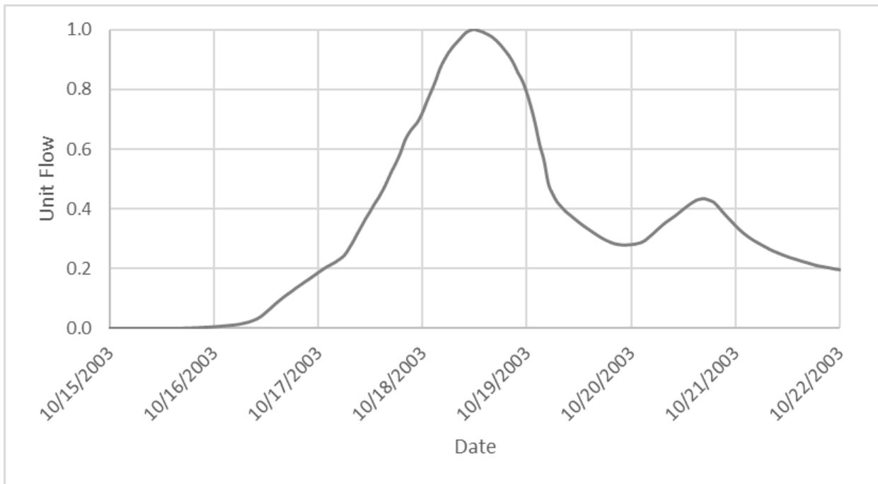
Figure 2.5 Unitless hydrograph developed from the 2003 flood of record at WSC 08MG005.
