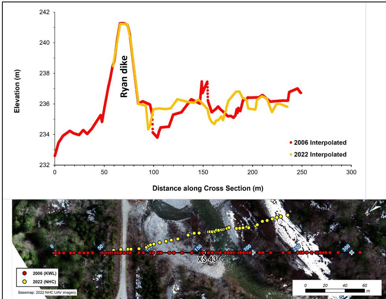
Figure 7.9 Cross-section 43 comparison.
