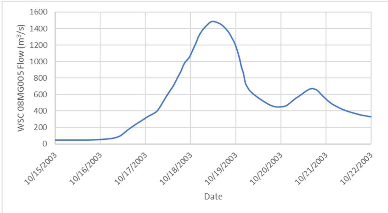
Figure 2.4 Hourly flow data for 2003 flood of record at WSC 08MG005.
