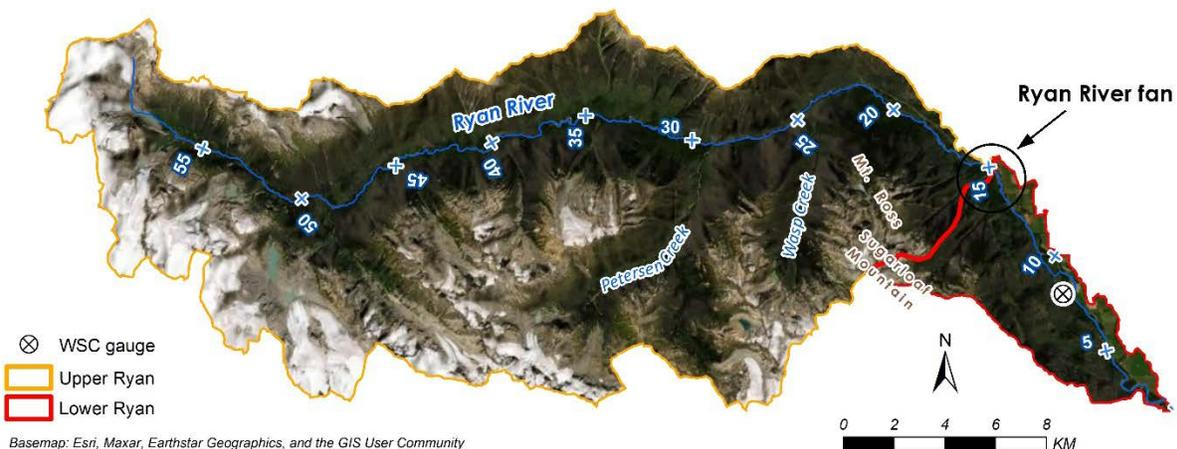
**Figure 3.1 Overview of the upper and lower Ryan River watersheds separated by the Ryan River fan. Crosses represent chainage markers, which are measured (in km) upstream of the mouth of the Ryan River.**
