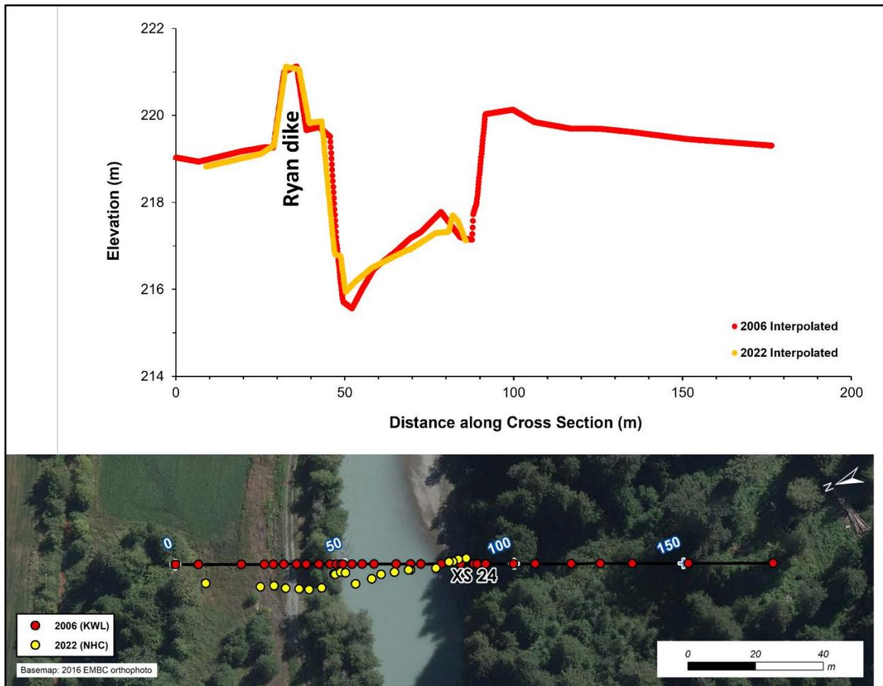
Figure 7.15 Cross-section 24 comparison.
