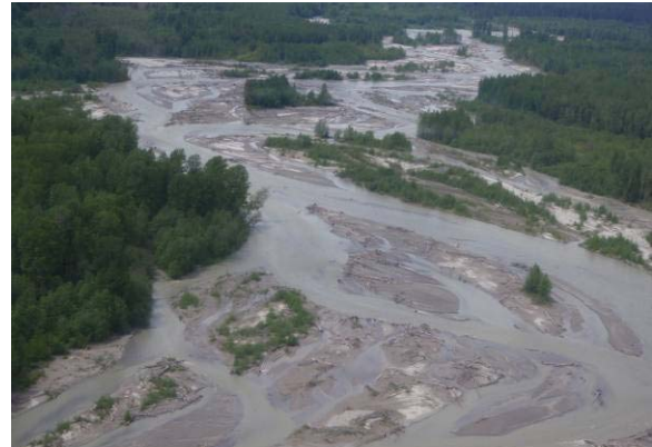
Photo F-8 Braided Channel Upstream of Forestry Bridge Showing Wood Storage in the Reach
